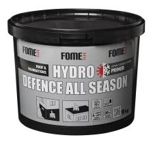
One-component bituminous primer for priming concrete surfaces before applying various bituminous water-proofing coatings. The primer is slightly modified with synthetic rubber and special additives that allow it to penetrate deeply into the base and strengthen it. The bituminous mixture can be used on slightly damp substrates, as well as on metal surfaces for corrosion protection. Suitable for use in all seasons.
